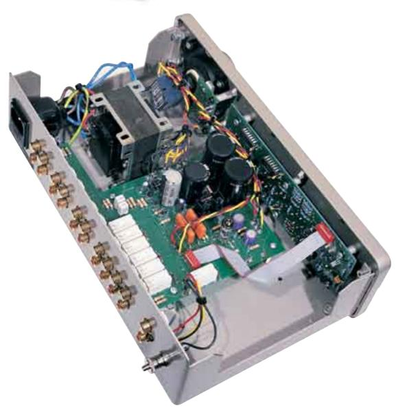
A completely new design, the QC-twenty-four pre amplifier is both neutral and detailed. Using a military specification 6111 valve, which is so reliable, it's hard-wired to the circuit board.
